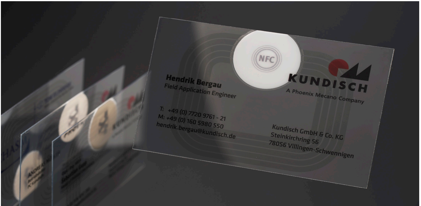
Fig. 5: Transparent NFC Tags. The high conductivity and yet high transparency enables one to produce transparent NFC tags. The Frequency of 13.56MHz is met although the coil resistance is much higher than aluminium etched antennas. The transparent NFC Tags can be comparable to printed NFC Tags using silver or copper inks, if the design is taking the novel material parameters of CNT + Metal Mesh into account.
